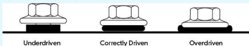
Figure 1: Correct tightening (driving) of fastener
