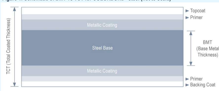
Figure 1: Schematic of BMT vs TCT for COLORBOND® steel (not to scale)
