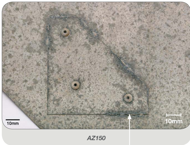
Dark areas indicate metallic coating corrosion originating from the cut-edge.
