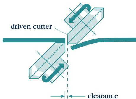
As with straight blade shearing, selection of correct clearance is necessary to obtain optimum edge quality and cutter life. Negative clearance,
