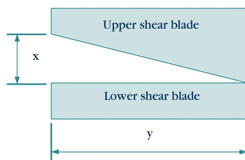
The angle known as shear angle, or as rake, is defined as the ratio  $x/y$ . Where shear is used, the workpiece is sheared progressively a little at a time, rather than instantaneously, as is the case with parallel blades. Rake, therefore, reduces the shearing force required to cut a sheet of a given thickness. The maximum rake in common use is 1/8. As rake is increased further, distortion of the workpiece increases, and the holddown forces necessary to avoid slippage increase.
