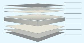
Finish Coat (Finish Coat + Primer = nominal  $33\mu m$ ) {Refer Notes 1, 5 & 6} Universal Corrosion Inhibitive Primer
