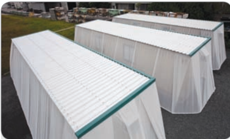
Figure 1 Test buildings with different roofing material (from left to right) ZINCALUME® steel, COLORBOND® Coolmax® steel in Whitehaven® and COLORBOND® steel in Surfmist®.
